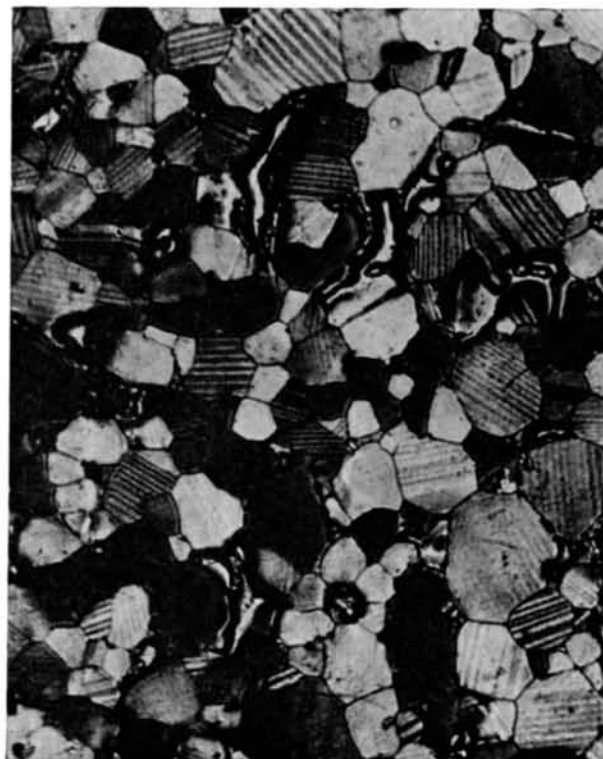
Fig. 1. Metallography of U 3 Si ( \times 500 ).
